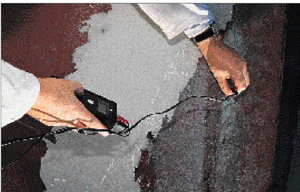
The ultrasonic gauge allows the surveyor to measure the thickness of the aluminum and steel hull plating.
