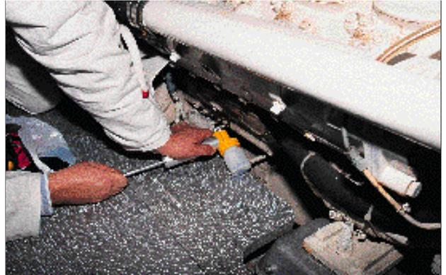
Oil samples are useful tools to assess the condition of engines.
