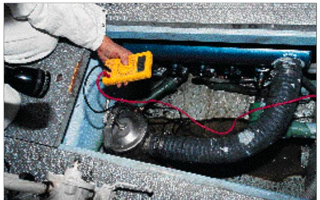
A voltmeter is used by the surveyor to check the efficiency of the bonding system and a reference cell.
