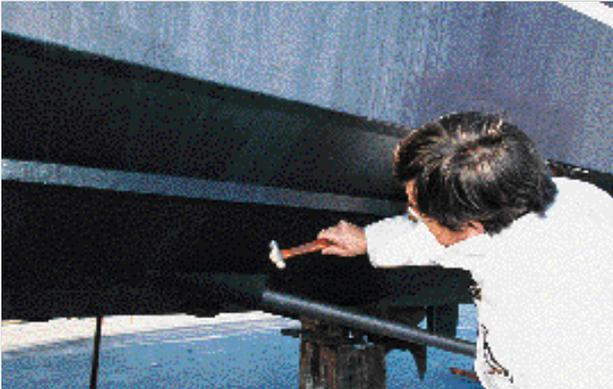
The surveyor uses a hammer to sound the hull shell and assess its condition.
