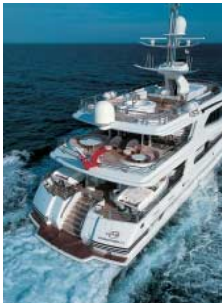
The question of stability must be taken into account when designing specifics such as a Jacuzzi or a Helideck.
