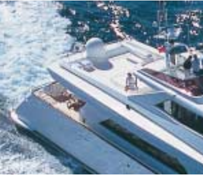
These liferafts are poorly located for rapid launch from the deck of this Guy Couach yacht.
