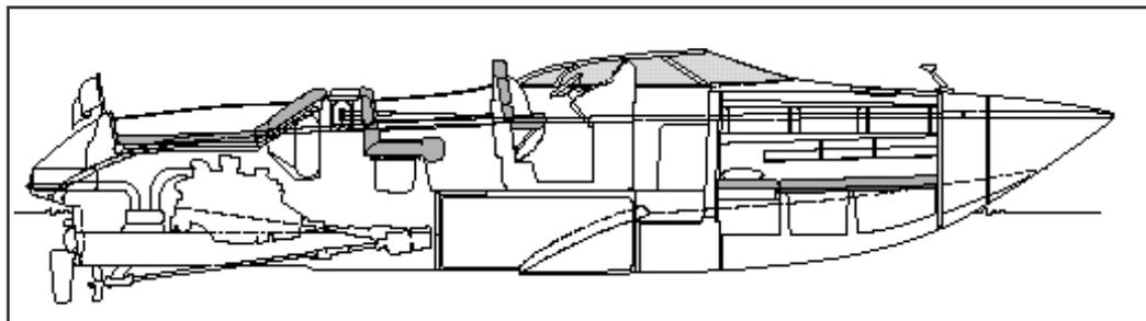
The V-drive allows the installation of the engine further aft while preserving the advantages of a conventional driveline.
