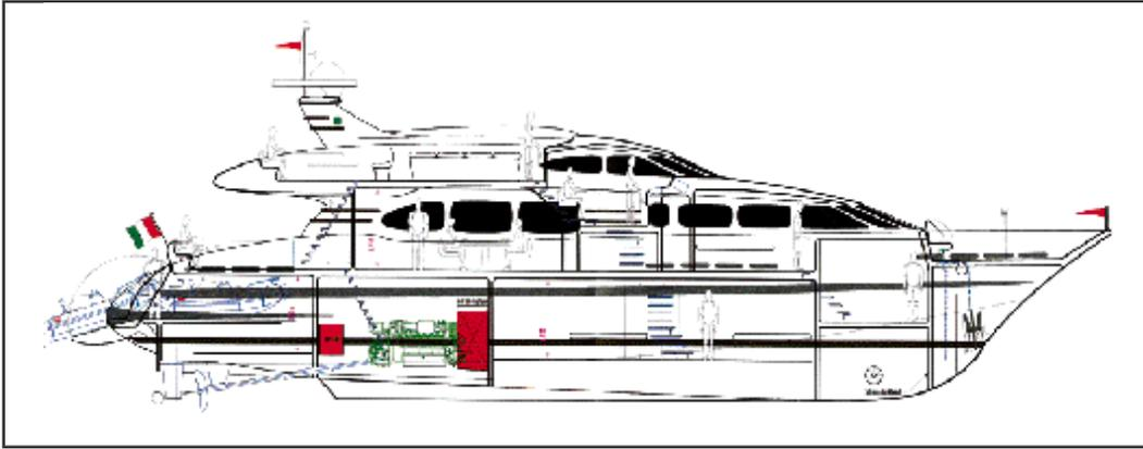
A direct line installation moves the engine and the center of gravity forward.
